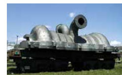
Steam Turbine Casing
