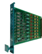
Prosafe-SLS Safety Instrumented System (Solid-state Logic Solver)
