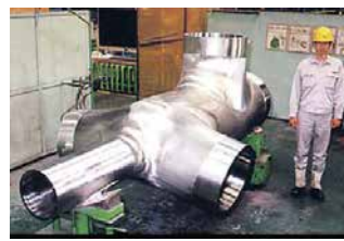
Primary Loop Piping
