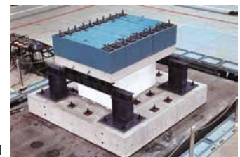
Shaking Test of NPP Concrete Wall
