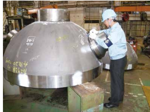
Inspection of welding
