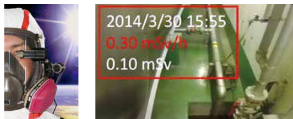
Example of indication in worker's view
