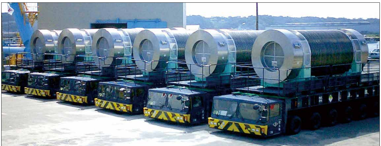
Speed Carrier (140tons)
