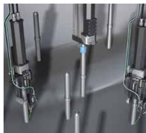
Portable Laser Peening Equipment
